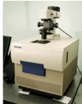
Image-based high content screening microscope with antibodies as orthogonal readout
